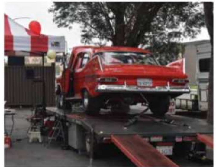
This Plymouth takes a dynamometer test, to show off its horsepower.
