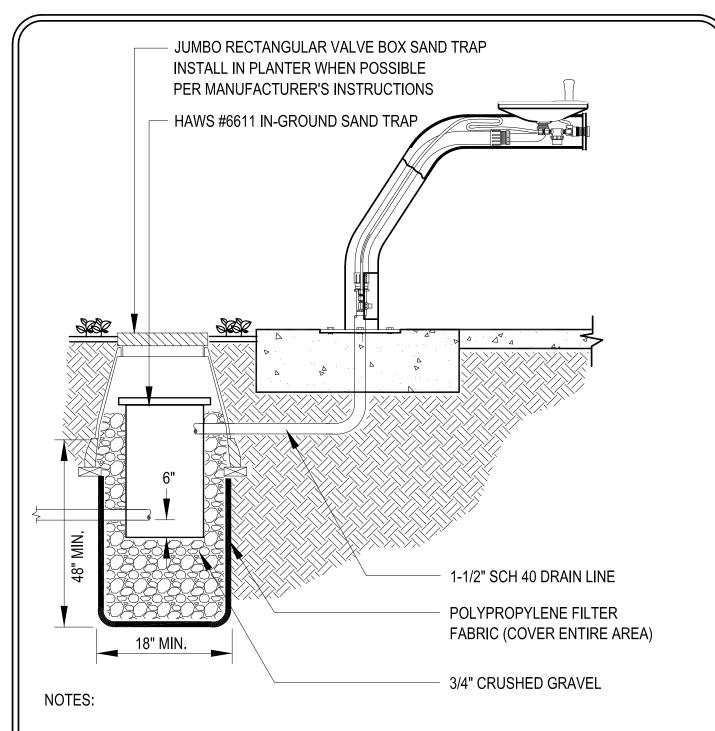
INSTALL DRAIN LINE PER PLAN, LOCAL CODES AND MANUFACTURER'S RECOMMENDATIONS DRAINLINE TO BE CONNECTED TO RESTROOM DRAIN OR OTHER BUILDING DRAIN WHEN POSSIBLE WHEN BUILDING DRAIN IS NOT AVAILABLE INSTALL DRAIN LINE IN 6'X6'X6' GRAVEL SUMP
