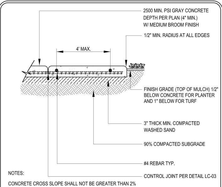
CONCRETE LONGITUDINAL SLOPE SHALL NOT BE GREATER THAN 5% WITHOUT HANDRAILS CONCRETE SHALL NOT BE FLATTER THAN 0.5% TO AVOID PONDING
