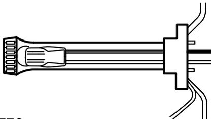
**STEP 5** POSITION WIRE CHANNELS AND SNAP INSULATOR TUBE COVER CLOSED
