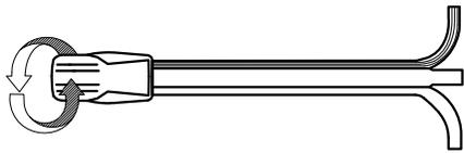
**STEP 3** APPLY SCOTCHLOK ELECTRICAL CONNECTOR AND TWIST IN A CLOCKWISE DIRECTION UNTIL TIGHT BUT DO NOT STRIP THREADS
