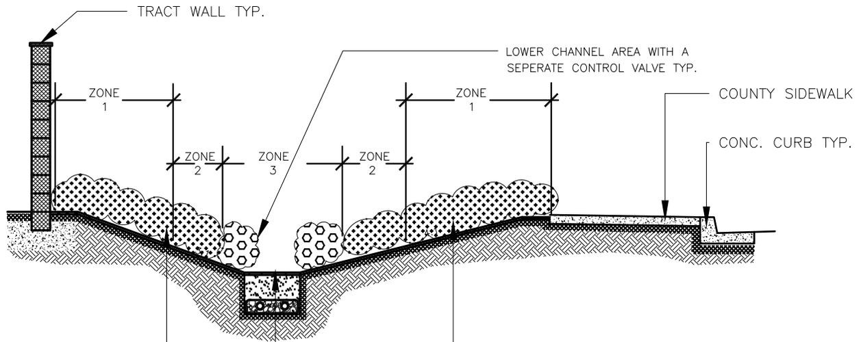
PARKWAY AREA IRRIGATED WITH THE TYPICAL LOW VOLUME CONTROL VALVE CONNECT LATERALS TOGETHER ON ONE CONTROL VALVE WHERE POSSIBLE.
