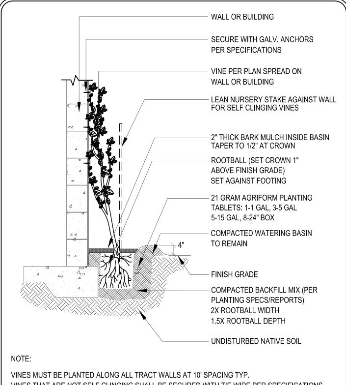
VINES THAT ARE NOT SELF CLINGING SHALL BE SECURED WITH TIE WIRE PER SPECIFICATIONS
