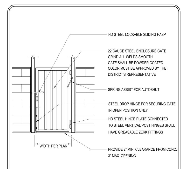
ALL STEEL FABRICATION SHALL RECEIVE 1 COAT EPOXY PRIMER AND 2 COATS OF EXTERIOR ENAMEL CONTRACTOR SHALL SUBMIT SHOP DRAWINGS AND COLOR SAMPLES FOR APPROVAL PRIOR TO CONSTRUCTION
