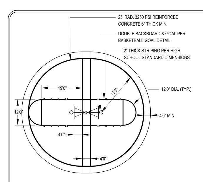
CONCRETE SHALL HAVE A HIGH POINT AT GOAL POST AND SLOPE TO PERIMETERS PER PLAN TO PROVIDE PROPER DRAINAGE (1% - 1.5% SLOPE REQUIRED)
