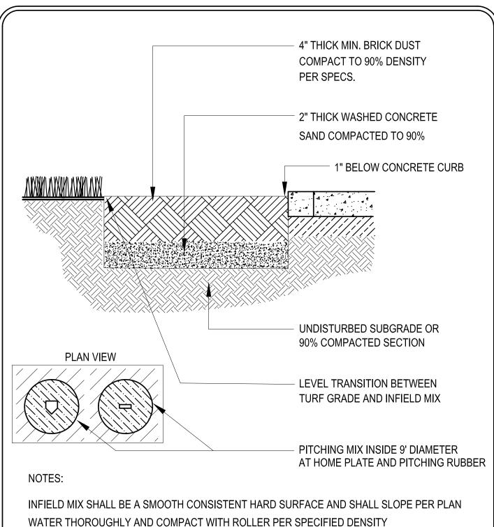
PROVIDE 9' DIAMETER PITCHING MIX 4" DEEP AROUND HOME PLATE AND PITCHING RUBBER
