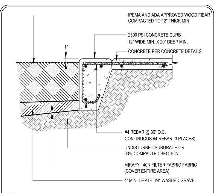
SUBGRADE FOR WOOD FIBAR SHALL SLOPE TO SUMP DRAINS PER PLAN FOR WATER RUNOFF PROVIDE 3/4" MIN. RADIUS AT CONCRETE EDGE
