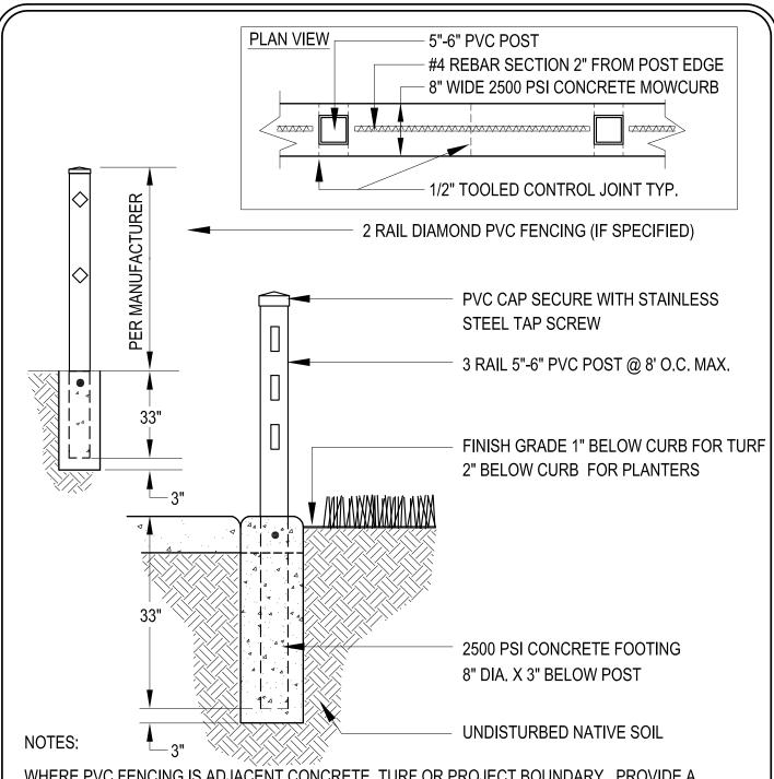
WHERE PVC FENCING IS ADJACENT CONCRETE, TURF OR PROJECT BOUNDARY, PROVIDE A CONCRETE MOWCURB ALONG FENCE LINE
