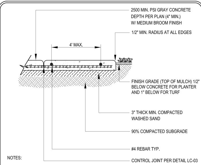
CONCRETE CROSS SLOPE SHALL NOT BE GREATER THAN 2%
