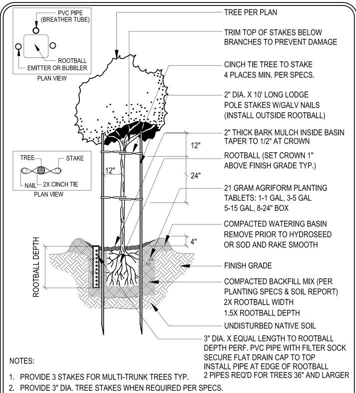
3. V.I.T. TWIST BRACES SHALL BE REQUIRED FOR PROJECTS WITH WINDY CONDITIONS
