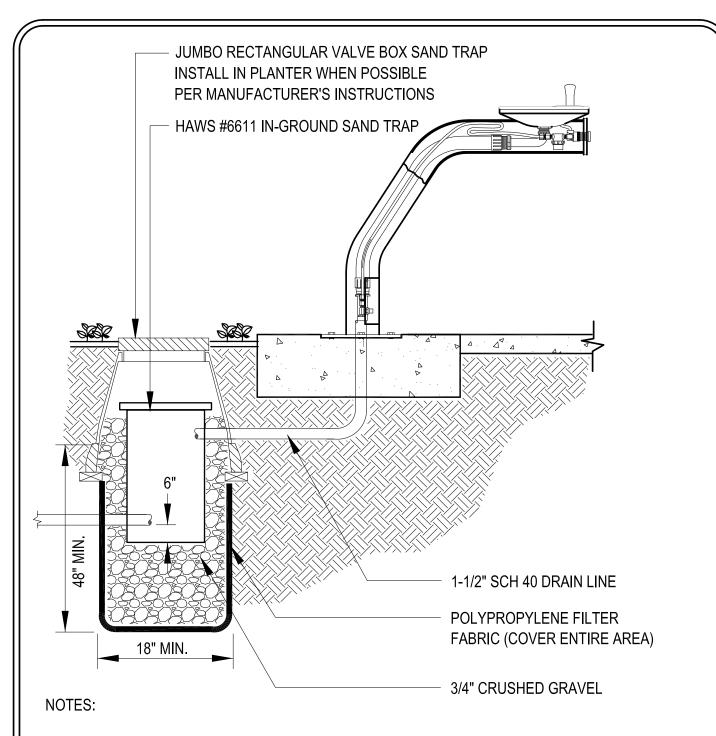
INSTALL DRAIN LINE PER PLAN, LOCAL CODES AND MANUFACTURER'S RECOMMENDATIONS DRAINLINE TO BE CONNECTED TO RESTROOM DRAIN OR OTHER BUILDING DRAIN WHEN POSSIBLE WHEN BUILDING DRAIN IS NOT AVAILABLE INSTALL DRAIN LINE IN 6'X6'X6' GRAVEL SUMP
