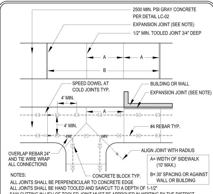
SAW CUTTING IN LIEU OF TOOLED JOINT MUST BE APPROVED IN WRITING BY THE DISTRICT PROVIDE 3/8" FELT EXPANSION JOINTS WHEN CONCRETE JOINS WITH WALL OR BUILDING PROVIDE 3/8" FELT EXPANSION JOINTS AT 30 FOOT SPACING TYP.
