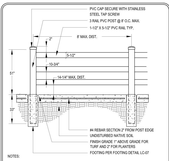
WHERE PVC FENCING IS ADJACENT CONCRETE, TURF OR PROJECT BOUNDARY, PROVIDE A CONCRETE MOWCURB ALONG FENCE LINE. REFER TO DETAIL LC-06 & 07 FOR FOOTING ELEVATION TOP OF FOOTING MUST BE AT ELEVATION TO ACCOMMODATE 6" DEEP FORM BOARDS AND CONCRETE MOWCURB TO BE POURED AFTER FOOTING AND POST INSTALLATION REFER TO DETAIL LC-09 FOR 2 RAIL DIAMOND STYLE PVC FENCING ALL FOOTINGS ARE SUBJECT TO SAME REQUIREMENTS INDICATED ON NOTE 4 OF DETAIL LC-06
