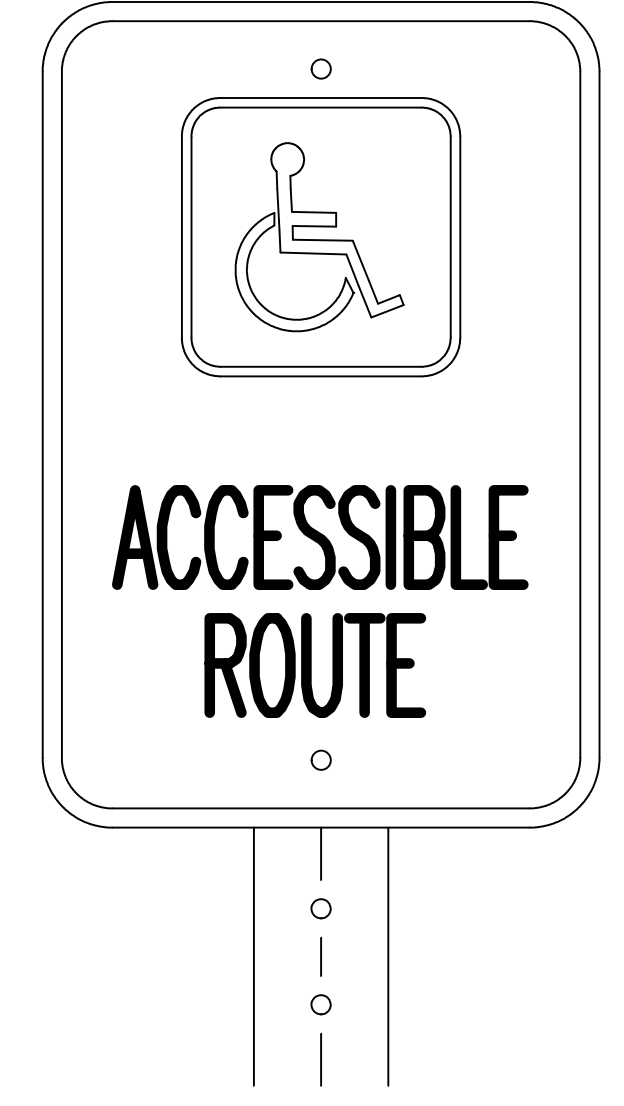
DETAIL 'A' ACCESSIBLE ROUTE SIGN NTS
