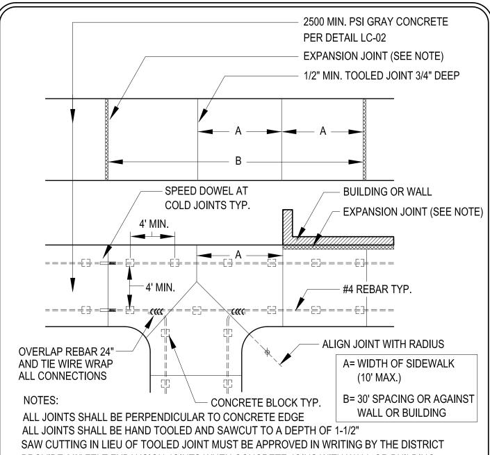
SAW CUTTING IN LIEU OF TOOLED JOINT MUST BE APPROVED IN WRITING BY THE DISTRICT PROVIDE 3/8" FELT EXPANSION JOINTS WHEN CONCRETE JOINS WITH WALL OR BUILDING PROVIDE 3/8" FELT EXPANSION JOINTS AT 30 FOOT SPACING TYP.
