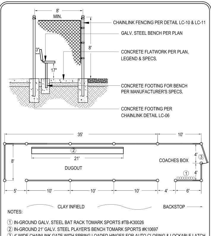
(3) 4' WIDE CHAINLINK GATE WITH SPRING LOADED HINGES FOR AUTO CLOSING & LOCKABLE LATCH
